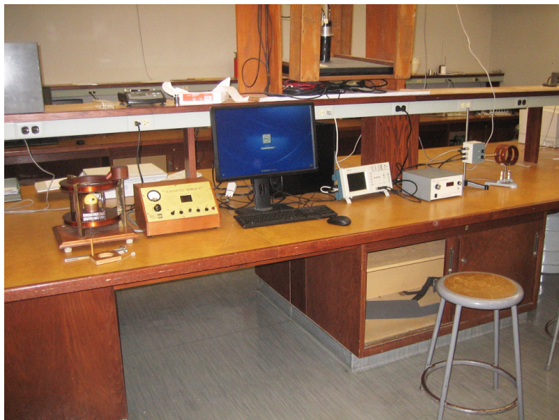
The apparatus: Teachspin Magnetic Torque apparatus, Daedelon Electron Spin apparatus, and digital oscilloscope. (Click on photo for a higher resolution view.)
