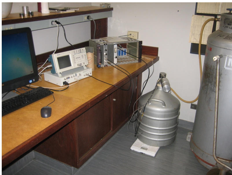
The apparatus: High purity germanium gamma detector in liquid nitrogen, NIM bin with high voltage power supply and amplifier, oscilloscope, pulse height analyzer, and computer. Gamma sources not shown. (Click on photo for a higher resolution view.)
