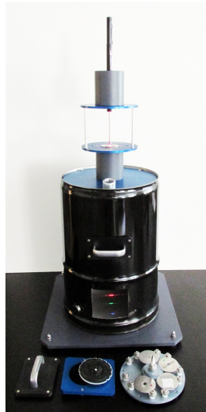
Apparatus for observing diffraction & interference patterns. For this image, the target is a 10 micron slit simultaneously illuminated by red, green and violet laser pointers.
